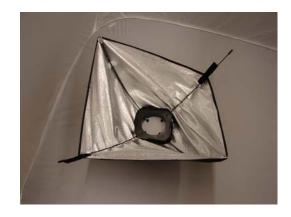
Close the end of the Velcro and the softbox assemble complete. You could add diffuser divider or simply add the diffuser cover out side of the softbox.
